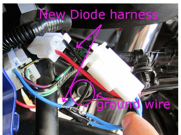
Pic of the new kit installed with the ground wire attached.
